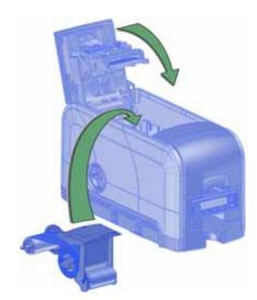
4. Close the printer cover. Press down on the ridges on the front of the cover to make sure that it latches completely on both sides.
