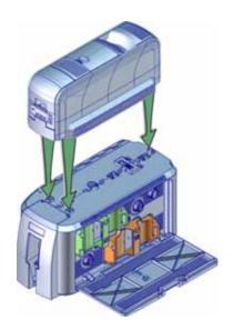
8. Connect the interconnect cable from the laminator to the lower port on the printer.
