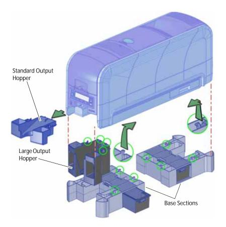
You can remove the standard hopper and attach the large output hopper without using tools.
