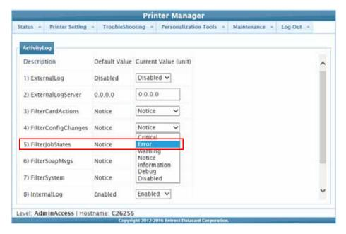
We recommend that you operate at all default logging settings to reduce unnecessary logging for typical printer operations.
