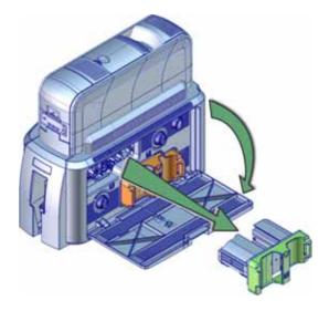
3. Push the release latch (a) and open the gate on the laminator cartridge (b).
